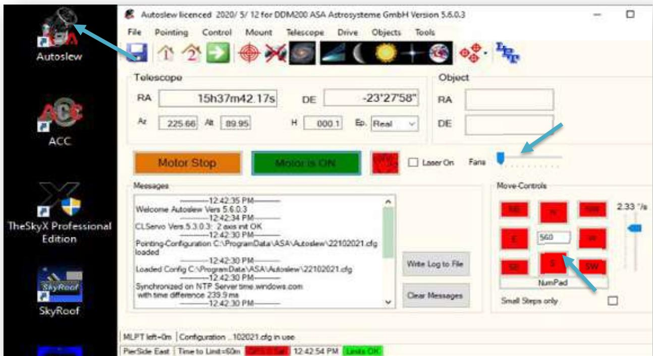
Start “Autoslew”, it will connect to the mount automatically, the motors are on by default.
